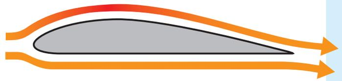
Airflow is slower over the lower surface and increases pressure
